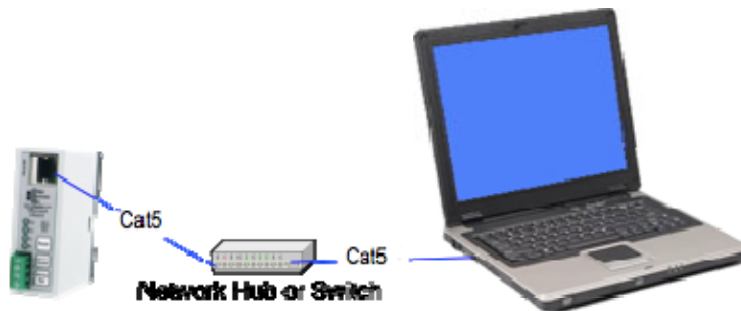
Fig.2.1: Ethernet setup with hub or switch
