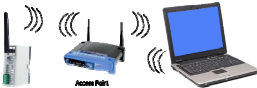
Fig.2.6: WiFi setup with access point and WiFi card on PC
