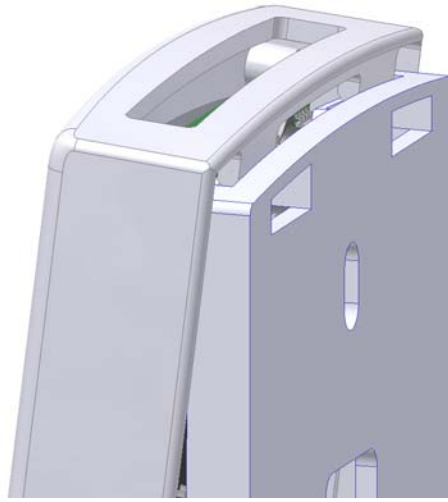
Figure 7.3.6, Align Cover Mounting Tabs with Base Mounting Slots
